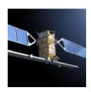
Sentinel-1 is a two satellite constellation with the prime objectives of Land and Ocean monitoring. The goal of the mission is to provide C-Band SAR data continuity following the retirement of ERS-2 and the end of the Envisat mission.
