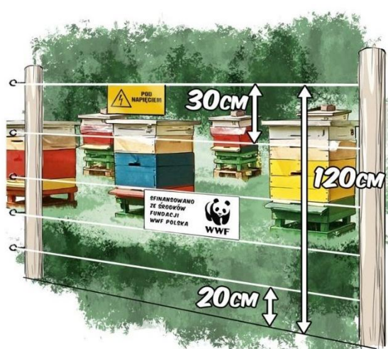
12. Figure - Schematic illustration about the installed protection measures in the Polish side of the East Carpathian pilot area
